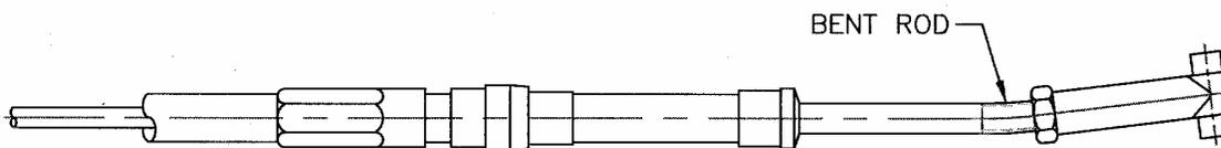
It is possible that a cable end may become bent either in transit during an installation or simply gets hit after it is installed. This, in fact, will also cause binding between the core rod and the sleeve.
